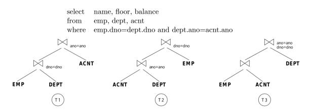
Figure 6: : Examples of join trees for the query; T3 has a cross product.
